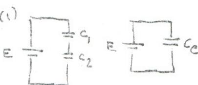
$$C_{\text{e}} = \frac{C_1 C_2}{C_1 + C_2} \quad C_{\text{e}} = \frac{2 \cdot 3}{2+3} = \frac{6}{5} = 1,2 \mu\text{F}$$
